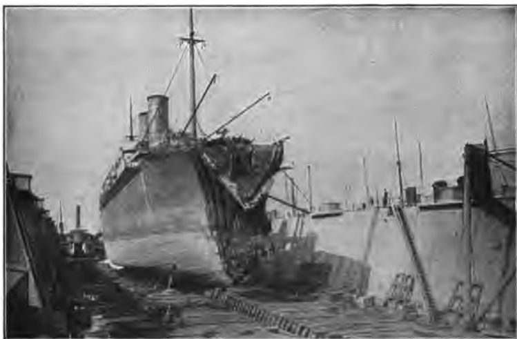
FIG. 147.—Steamer in dry dock at Fifty-fifth Street, Brooklyn, after collision off Massachusetts coast. Steel construction preventing shivering of ship and water-tight compartments prevented filling and sinking. Ships are sometimes built in dry docks like this one.
